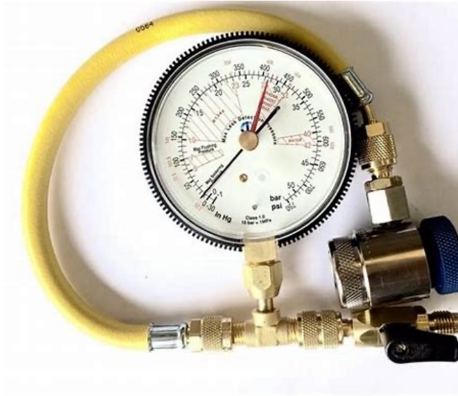
Leak detection gauge
