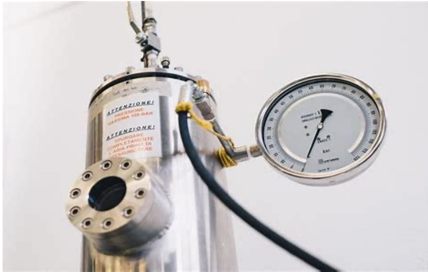
Hydrostatic pressure testing
